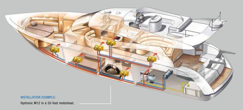
Fan radiator Convector Radiator Calorifier T-piece Safety group Overflow valve Filling and drain Fuel metering pump valve Tank connection Hull fitting Combustion air pipe with silencer Exhaust system with silencer Boat tank
