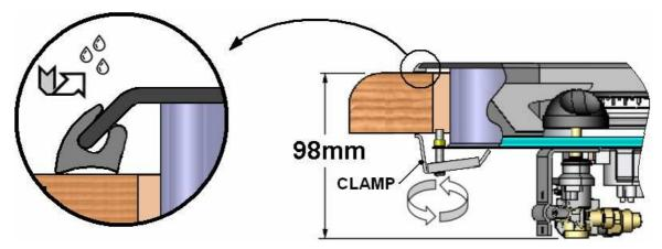
FIG. 7 SERIES 160,162,164 & 167 INSET HOBS (Flush Mount Seal)
