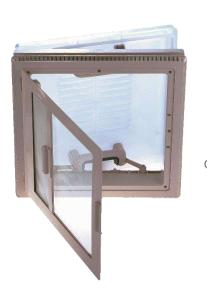
400 x 400 mm Aperture Roof thickness 24-56 bzw. 42-70 mm Corner radius 23 mm Site dome 470 x 470 mm Height over roof 91 mm Ventilation 150 / 30 cm<sup>2</sup> Weight 2.5 kg 470 x 470 x 14 mm Size inner frame Outer frame material Polypropylene Dome material Polypropylene 130 km/h Speed limit ECE R43 -019649 Authorization
