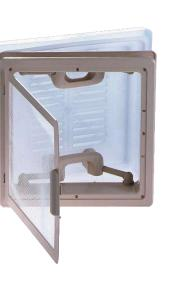
280 x 280 mm Aperture Roof thickness 24-46 bzw. 42-72 mm Corner radius 18 mm Site dome 330 x 330 mm Height over roof 78 mm Ventilation 60 cm<sup>2</sup> Weight 1.3 kg 314 x 314 x 9 mm Size inner frame Outer frame material Polypropylene Dome material Polypropylene 130 km/h Speed limit Authorization ECE R43 -019649
