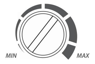
Please note that the appliance can only be switched on when the thermostat setting is higher then the room temperature.
