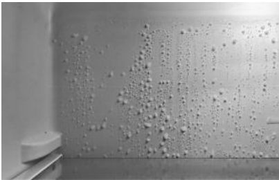
Rear wall showing Ice Droplets during Cooling Phase.
