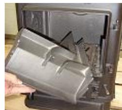
7. Remove the rear heat shield using a 10mm spanner or socket wrench
