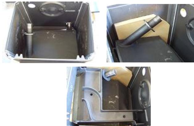
12. Bolt the top plate back into position, this is best achieved through the top flue outlet.
