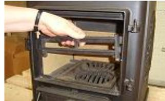
3. Remove side brick by lifting the baffle plate and rotating each brick in turn towards the centre of the stove; the bricks can then be removed diagonally through the door aperture. The back brick can now be easily removed from the stove
