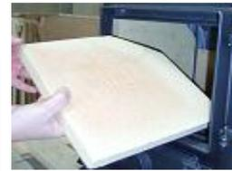
4. Rotate the cast iron baffle plate through 90° and remove
